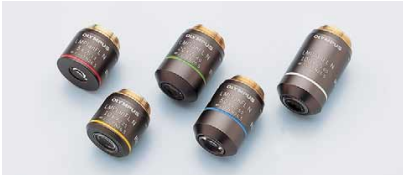
LMPLFLN (-BD) Plan SemiApochromat series The LMPLFLN (-BD) series provides more free space between the objective lens and the specimen than other Plan SemiApochromatic objective lens series so that it can prevent from collision between objective lens with the stepped specimen. Since exit pupil positions from 5x through 100x are standardized, no switching of the DIC prism lever position is necessary when the objective lens power changes . Use the BD series in brightfield and darkfield observation.
