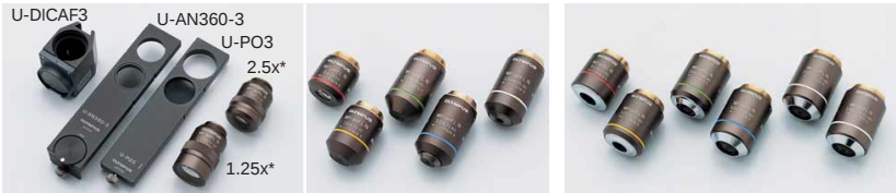
MPLFLN (-BD) Plan SemiApochromat series These Plan SemiApochromat objective lenses completely eliminate chromatic aberration at high level, which is perfect for a wide range of microscopic methods including brightfield darkfield, fluorescence, Nomarski DIC and simple polarized observation. Since exit pupil positions from 5x through 150x are standardized, no switching of the DIC prism lever position is necessary when the objective lens power changes. Use the BD series in brightfield and darkfield observation. * High contrast images are obtained at 1.25x or 2.5x observation combining with both analyzer (U-AN360-3) and polarizer (U-DICAF2 for MX61, U-PO3 for MX51)
