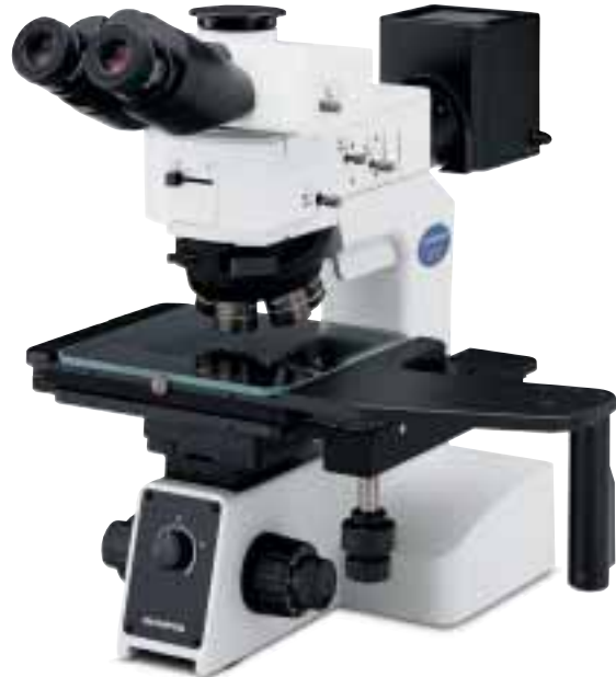
Reflected/transmitted light configuration with 150mm stage MX51+BX-RLA2+MX-SIC6R2+BH3-SPG6+MX-TILL
