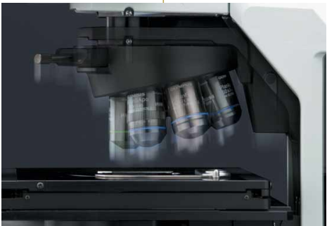
Microscope Frame Equipped with Motorized Focus and Field Diaphragm This unit incorporates a high-speed, high-precision motorized focusing nosepiece with 0.01 \mu\text{m} resolution and 20 mm vertical strokes. The field diaphragm adjustment of transmitted light is also motorized.
